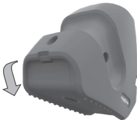
When the battery indicator **3** flashes red, the batteries must be replaced.
