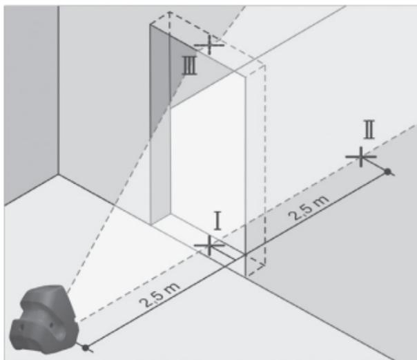
Mark the centre of the vertical laser line at the floor of the door opening (point I), at a distance of 5 meters beyond the other side of the door opening (point II) and at the upper edge of the door opening (point III).
