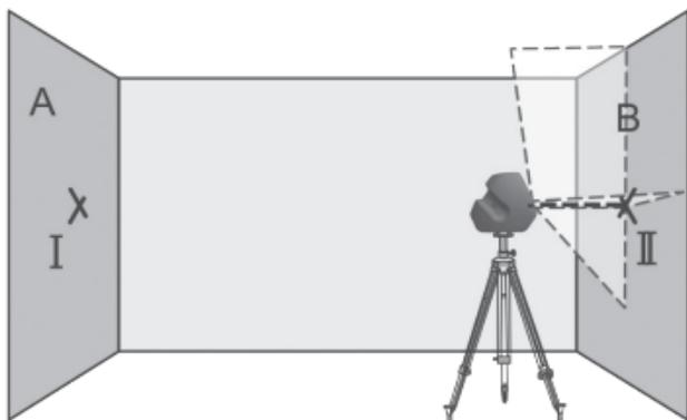
Without changing the height, turn around the instrument by 180°. Direct it against the wall A such a manner that the vertical laser line runs through the already marked point I. Allow the instrument to level in and mark the cross point of the laser lines on the wall A (point III).
