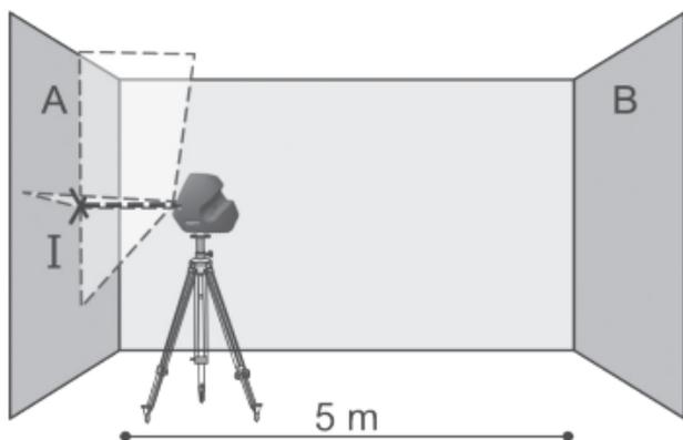
Turn the instrument by 180°, allow it to level in and mark the cross point of the laser lines on the opposite wall B (point II).
