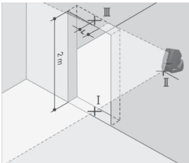
The difference  $L$  between point III and the centre of the laser line at the upper edge of the door opening results in the actual deviation of the instrument from the vertical plane.
