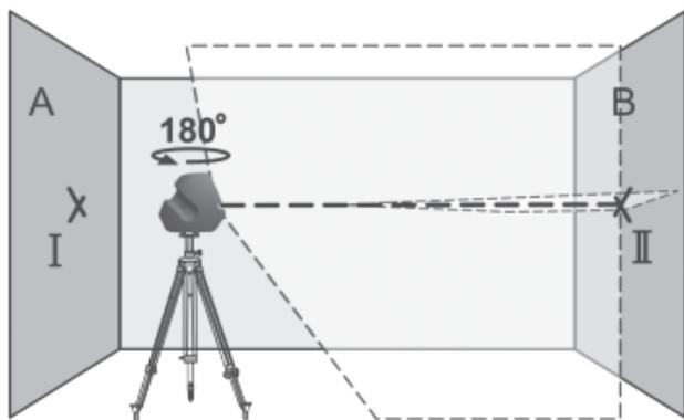
Without turning the instrument, position it close to wall B. Switch the instrument on and allow it to level in.
