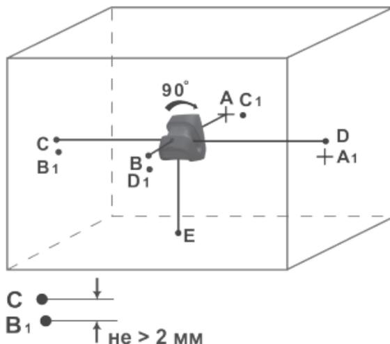
If the value is larger than 2 mm, the instrument must be returned to CONDROL service centre.
