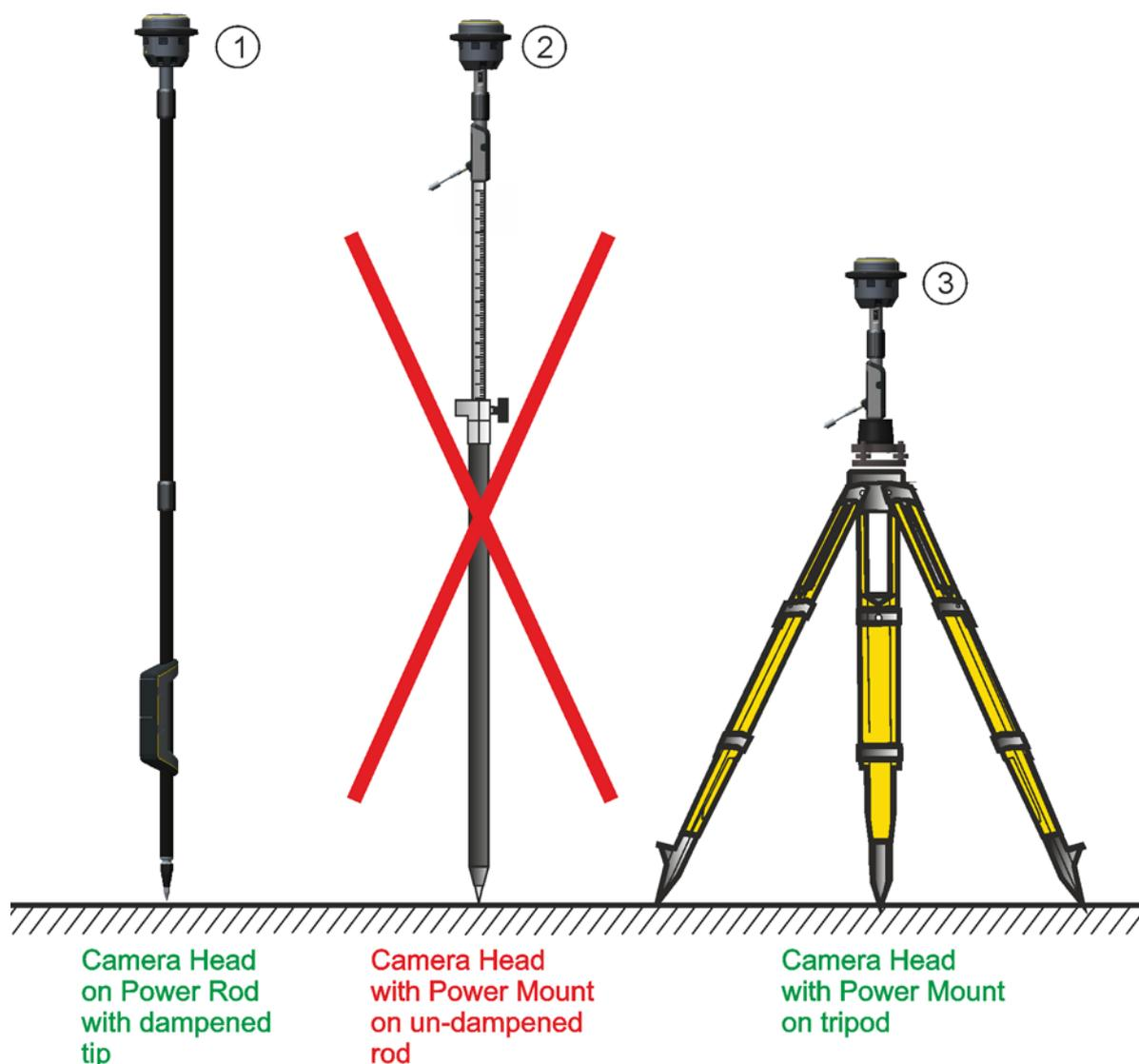
Figure 2.12 Correct and incorrect set up of the camera head
