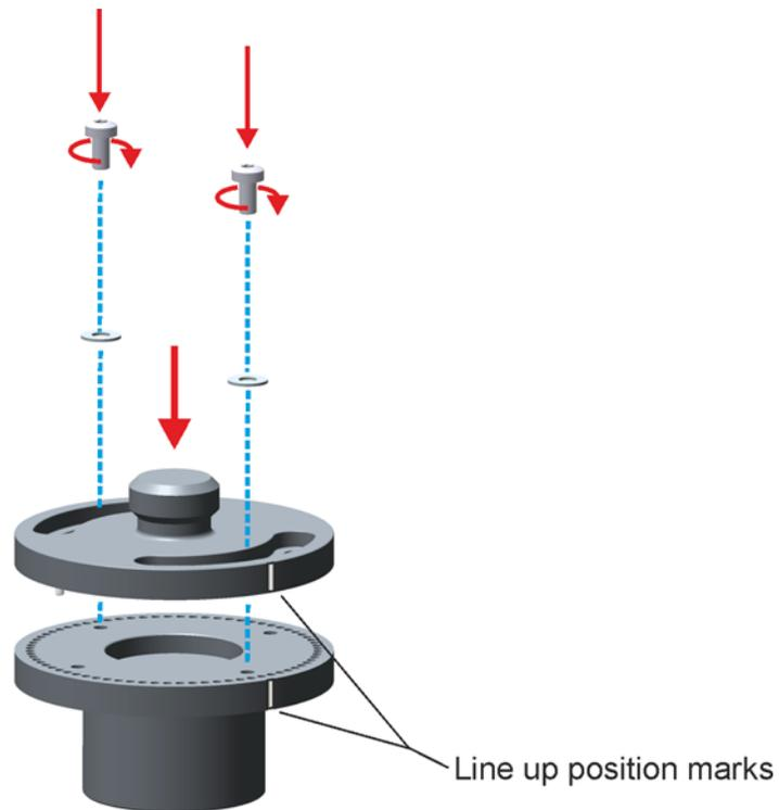
Figure 2.43 Putting the adapter parts together
