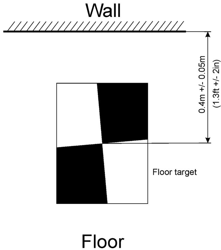
Figure 3.63 Floor target set up
