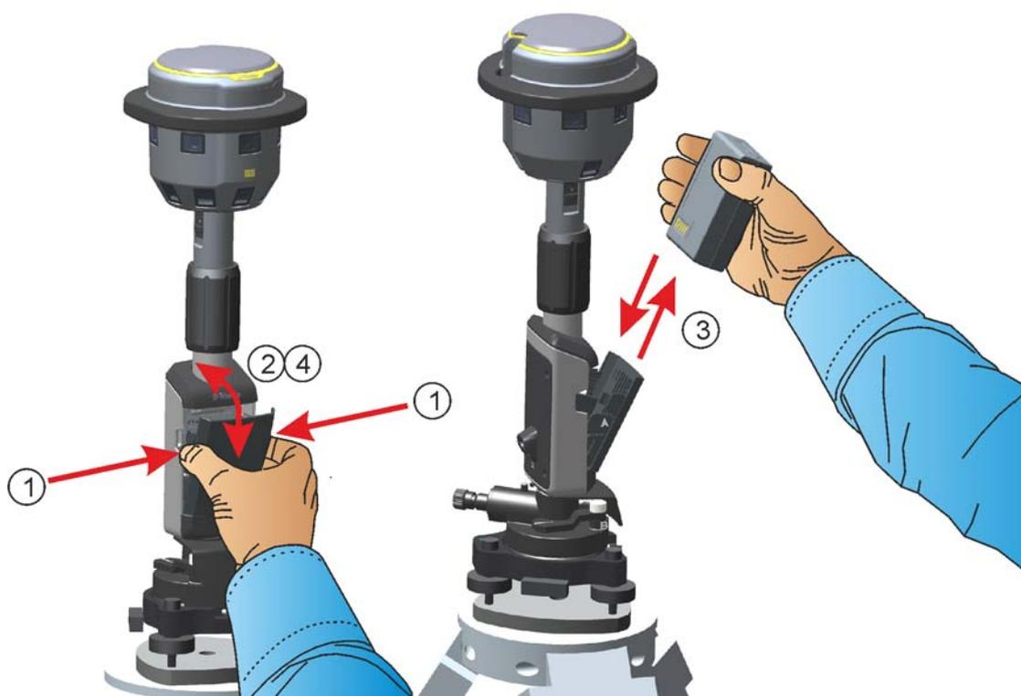
Figure 2.31 Inserting a battery in the power mount battery compartment.
