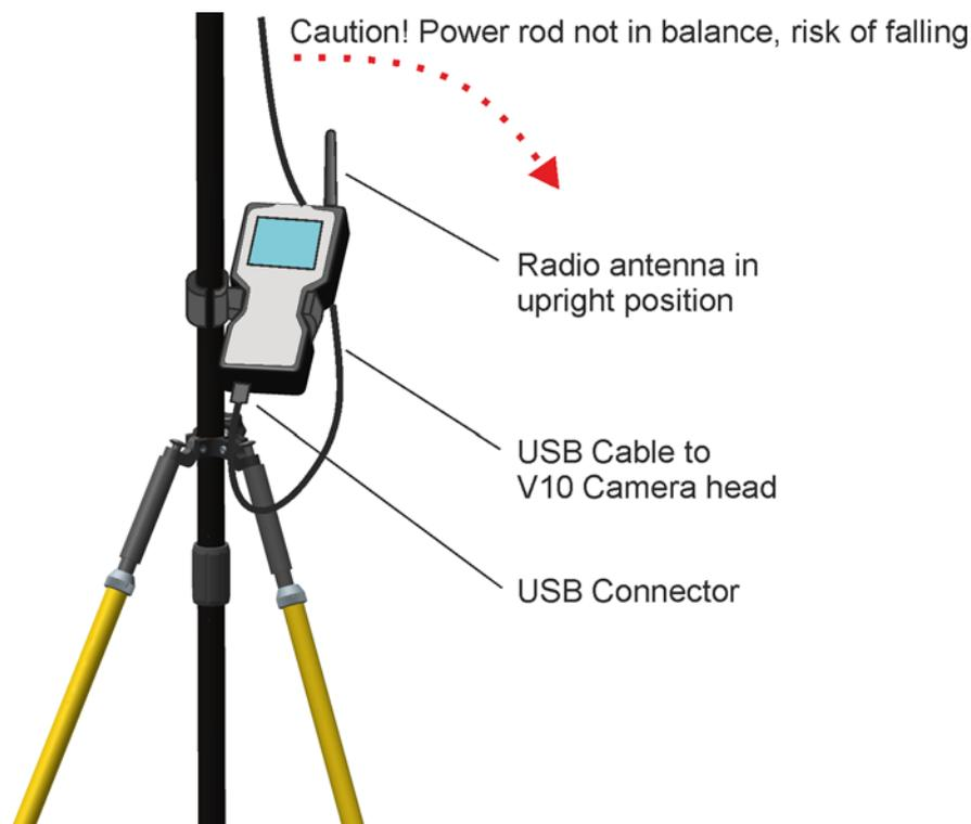
Figure 2.25 TSC3 Controller mounted on power rod
