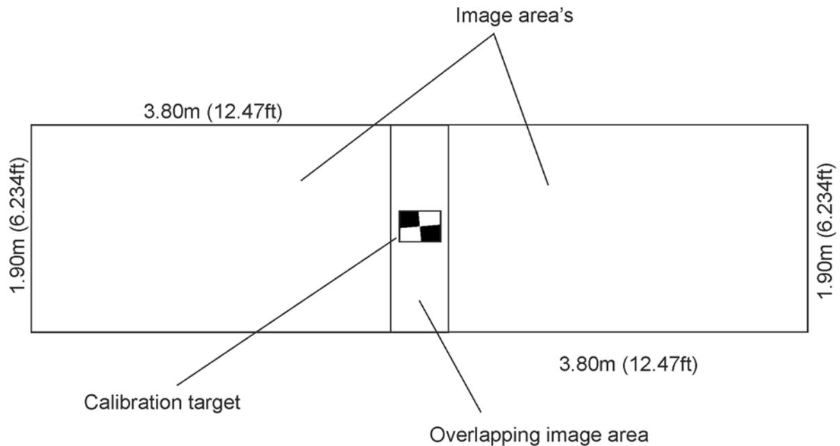
Figure 3.59 The size of the image area is about 3.80m wide and 1.90m high on the 2m calibration check distance
