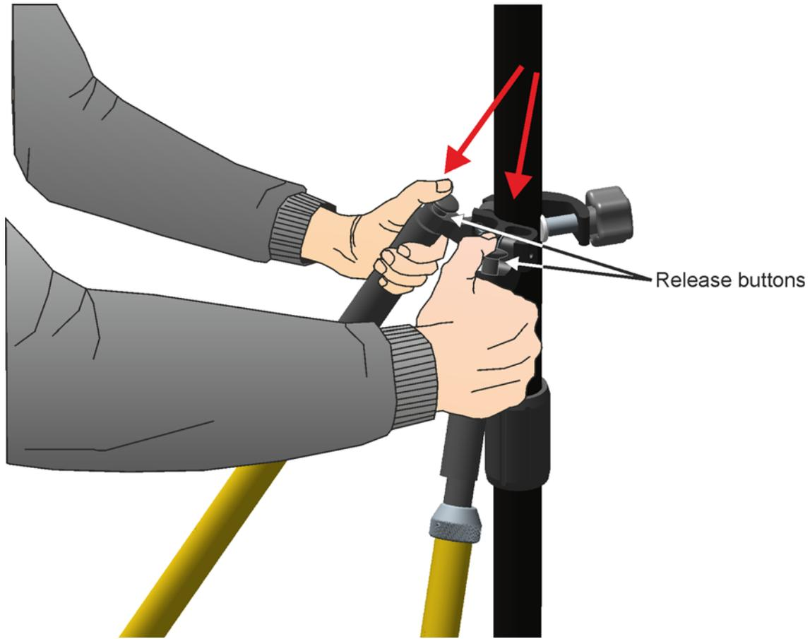
Figure 2.20 Adjusting the length of the bi-pod legs
