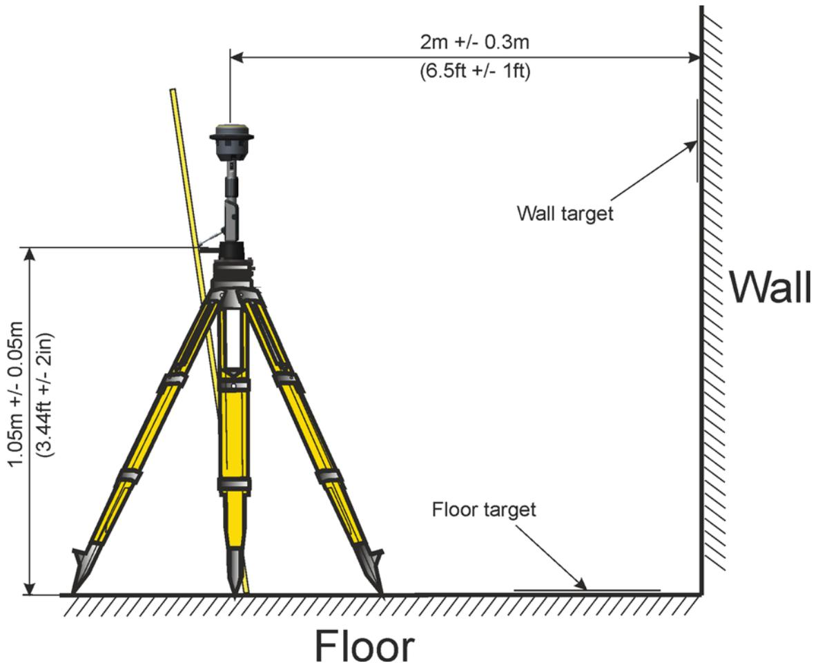
Figure 3.64 Camera head set up
