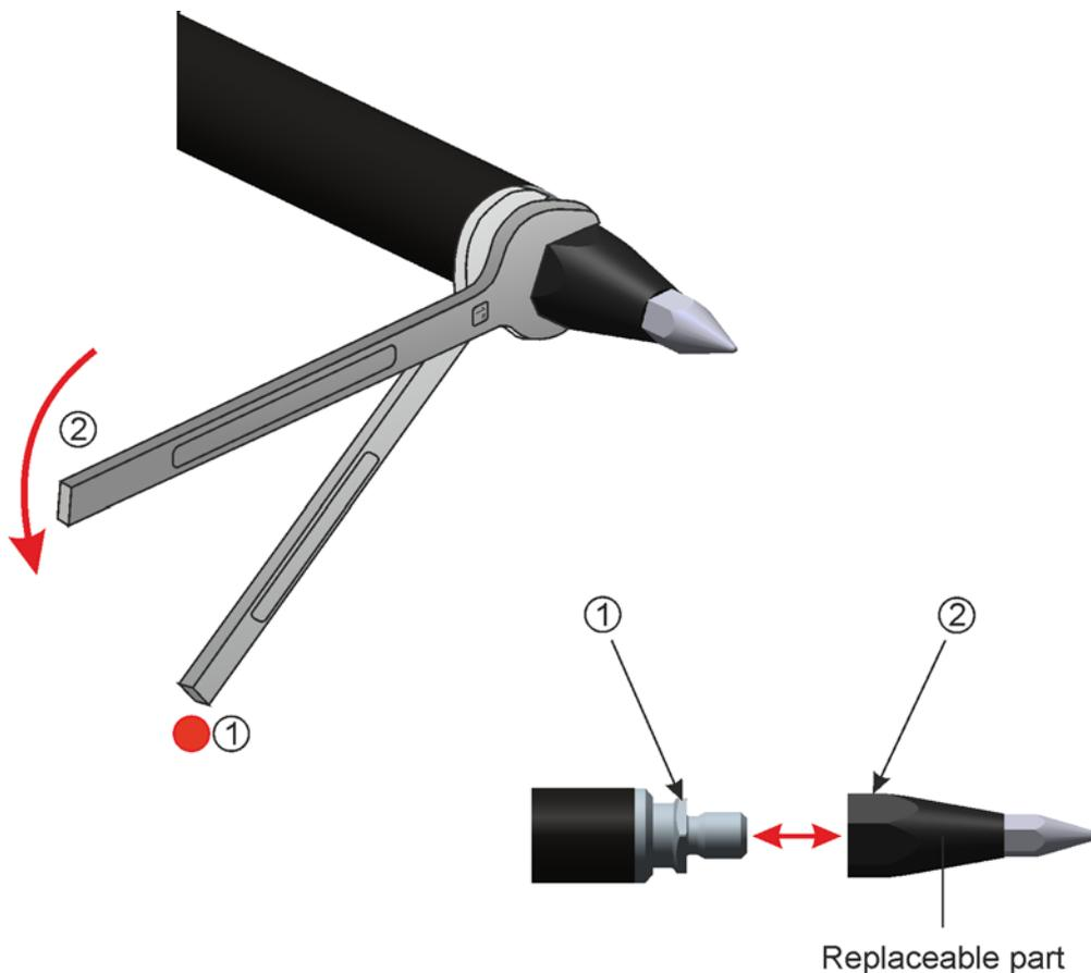
Figure 3.65 Replacing the power rod tip
