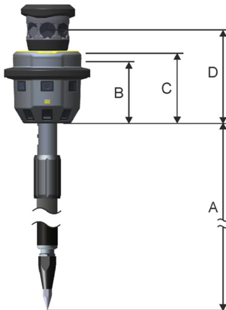
Figure 2.51 Instrument heights on power rod with Prism 360 1 inch p.c.2mm
