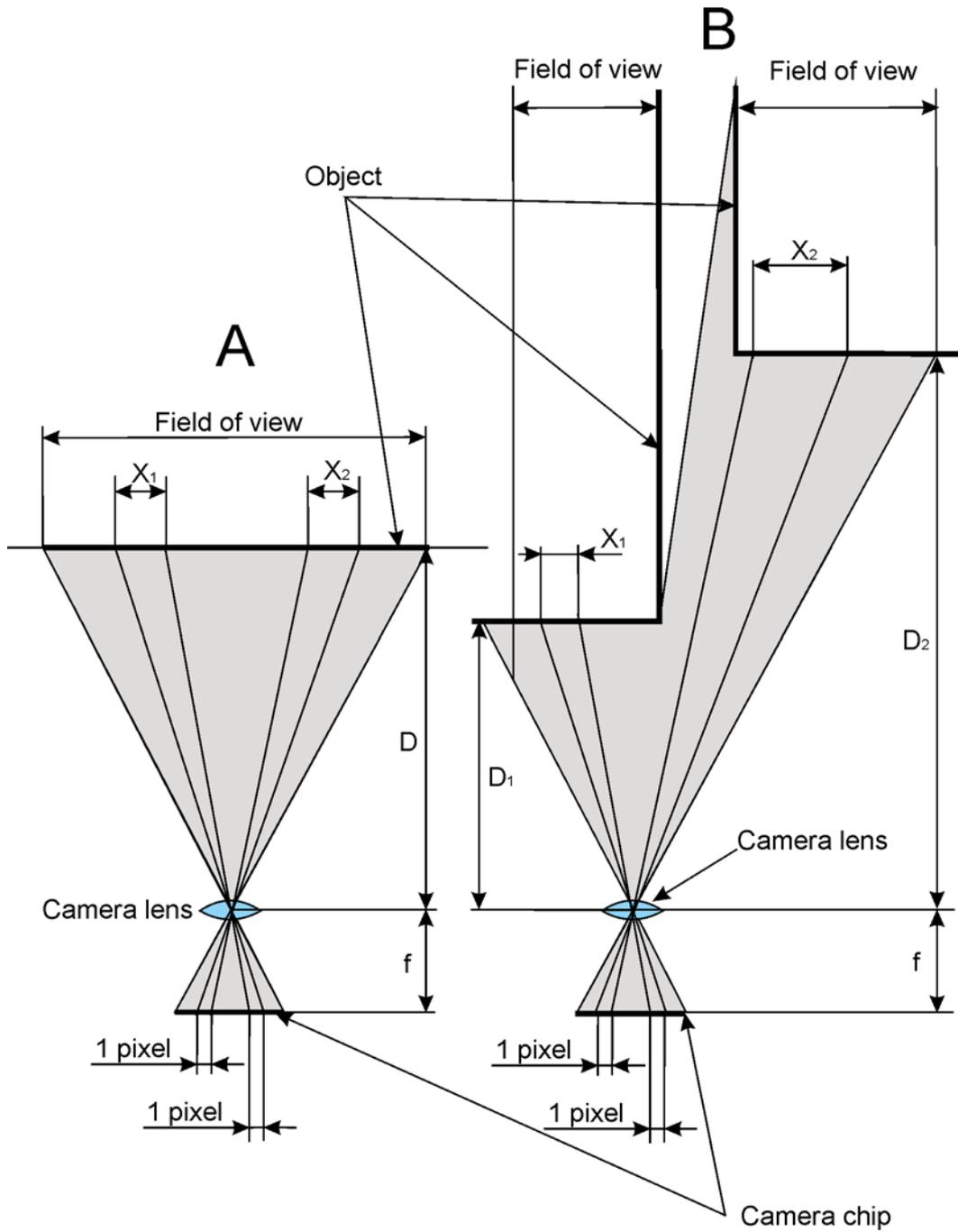
Figure 4.5 Difference in accuracy in proportion to the distance in an image due to multiple objects at different distances from the instrument.
