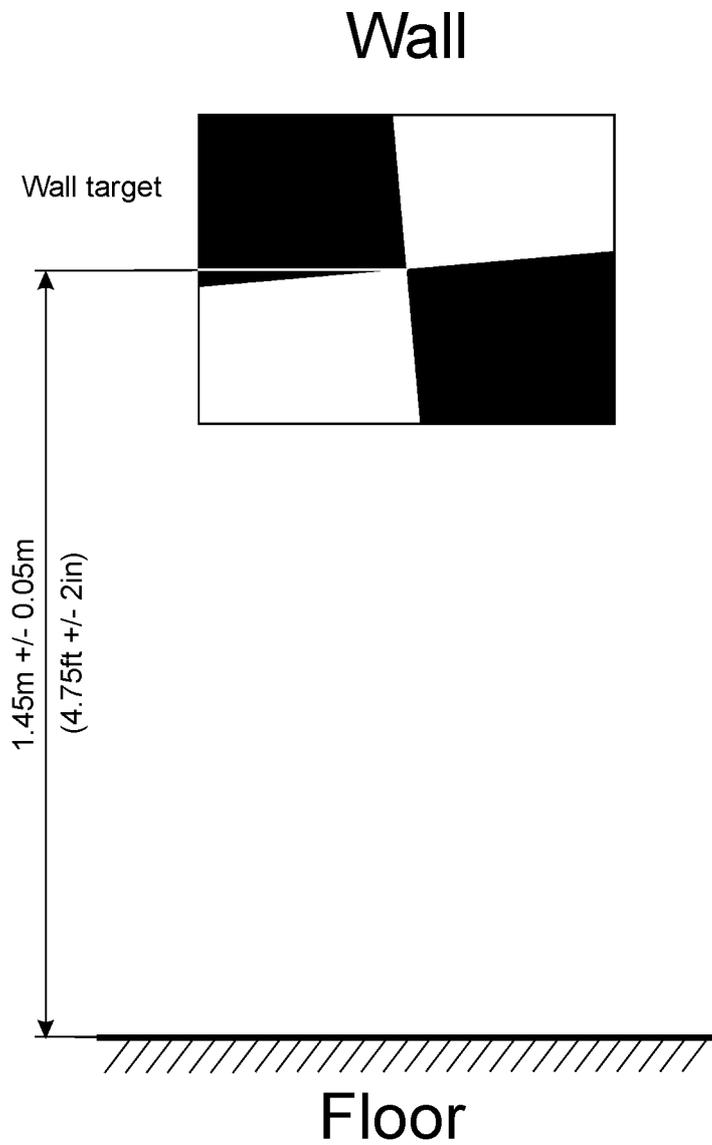
Figure 3.62 Wall target set up
