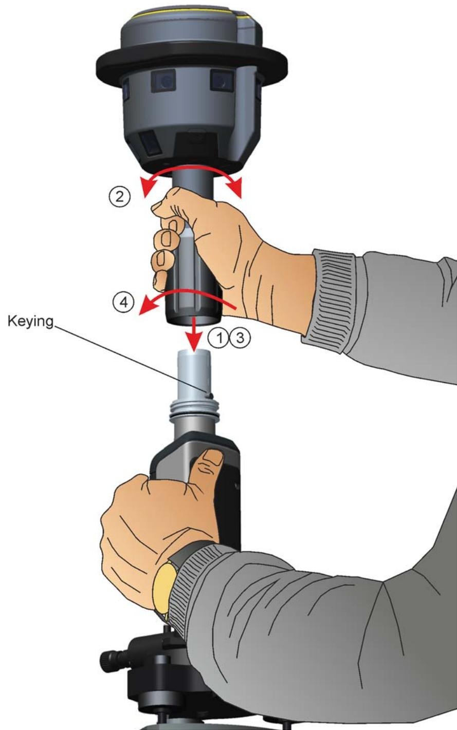
Figure 2.29 Connecting the camera head to the power mount
