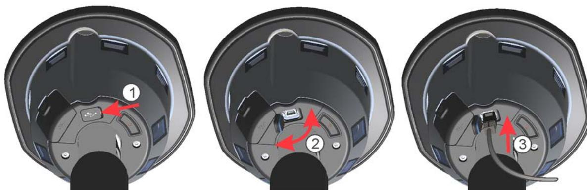
Figure 2.48 Connecting the 1.5m cable with mini USB connector
