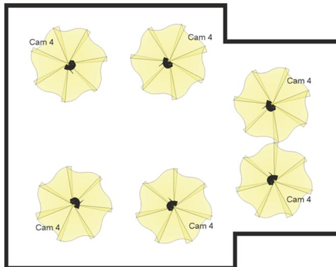
Figure 4.7 Several panoramas made to obtain the same photogrammetry measurement accuracy.
