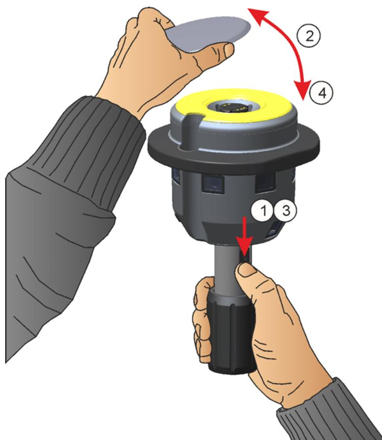
Figure 2.34 Removing the quick release cover
