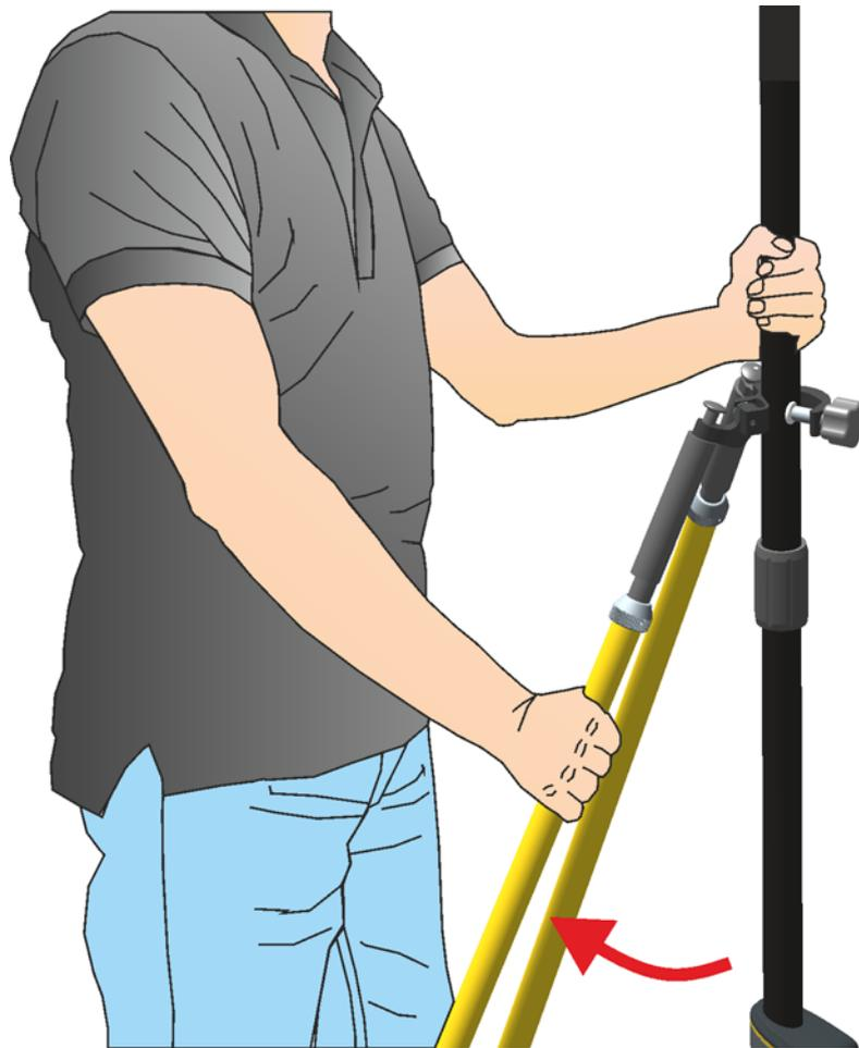
Figure 2.19 Pulling out the bi-pod legs
