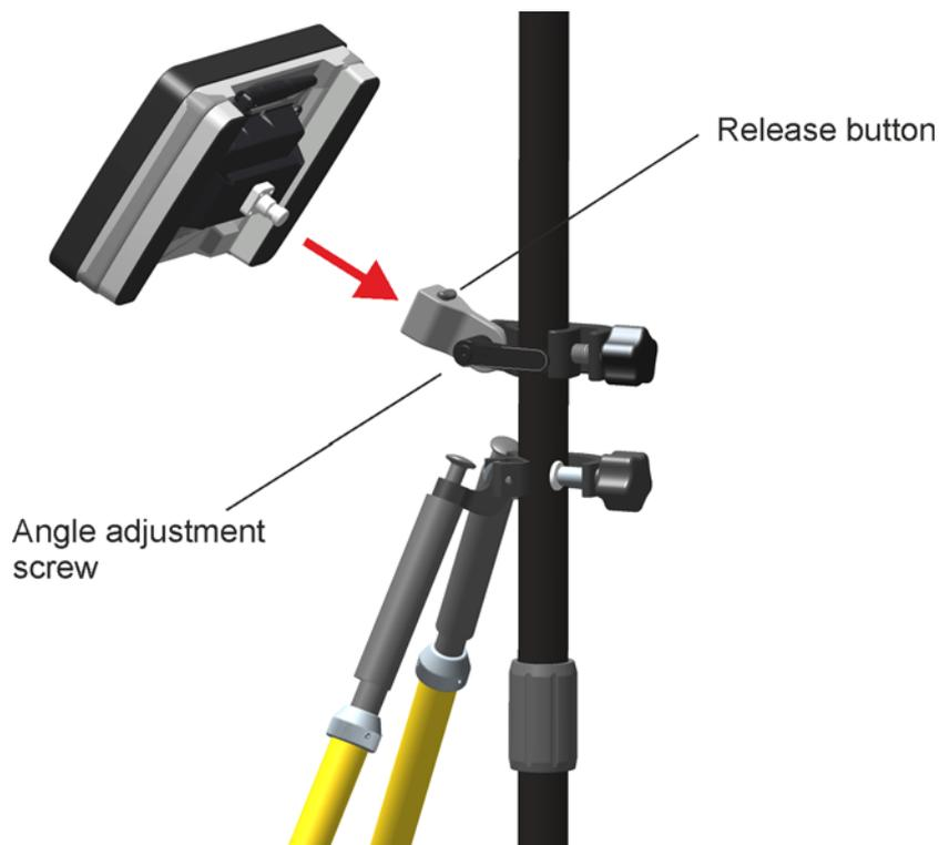
Figure 2.22 Mounting the tablet PC
