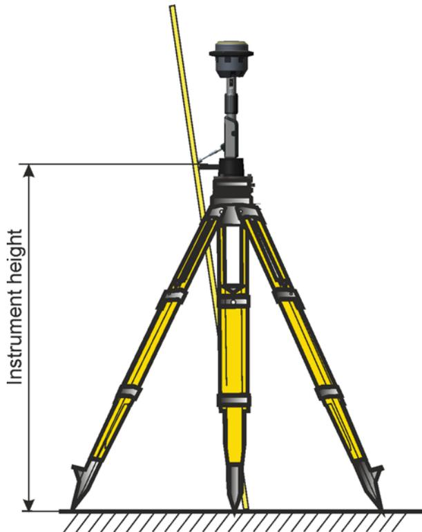
Figure 2.52 Instrument height with power mount
