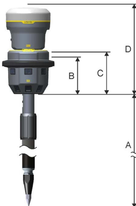
Figure 2.49 Instrument heights on power rod with R10 GNSS receiver
