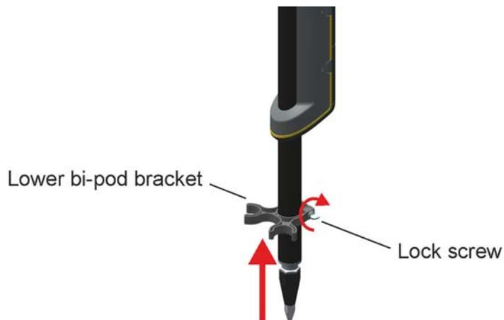
Figure 2.17 Mounting lower bi-pod bracket
