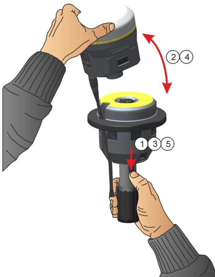
Figure 2.36 Connecting a Trimble R10 GNSS Receiver to the Trimble V10 Imaging Rover
