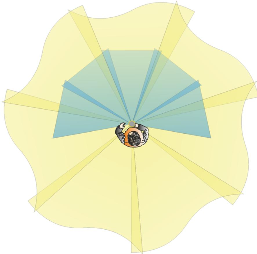
Figure 4.1 Horizontal field of view. Upper camera row yellow and lower camera row blue.
