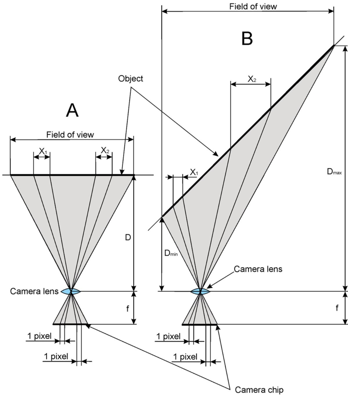
Figure 4.4 Difference in accuracy in proportion to the distance in an image due to object being in an angle in relation to the camera chip.
