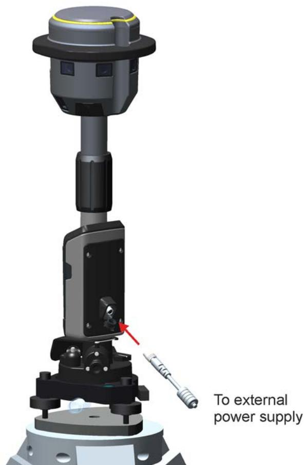
Figure 2.32 Connecting external power supply.
