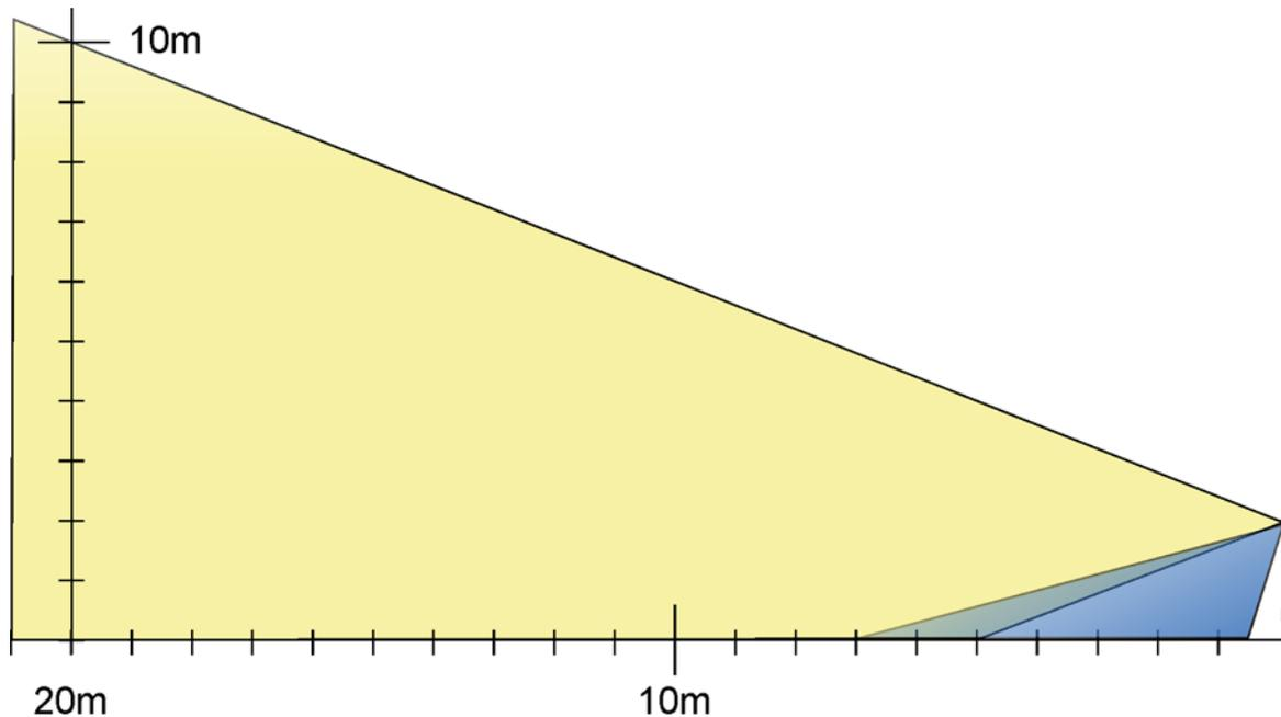
Figure 4.2 Vertical field of view. Upper camera row yellow and lower camera row blue.
