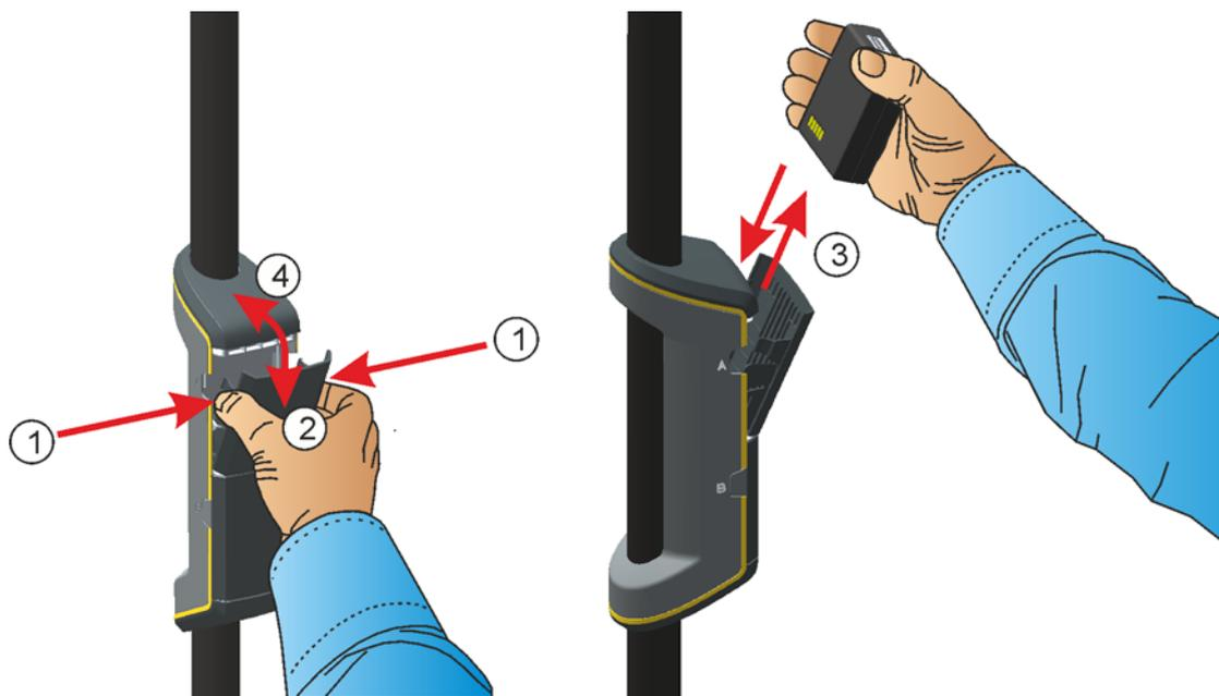
Figure 2.26 Inserting a battery in the power rod's battery compartment A.
