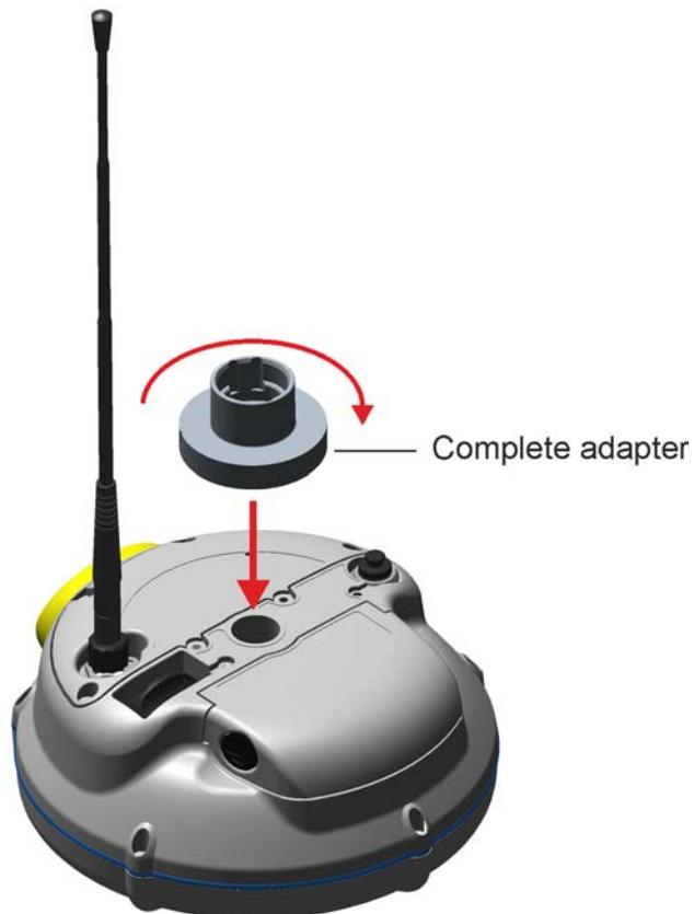
Figure 2.44 Fitting the QR to 5/8" adapter to the GNSS receiver
