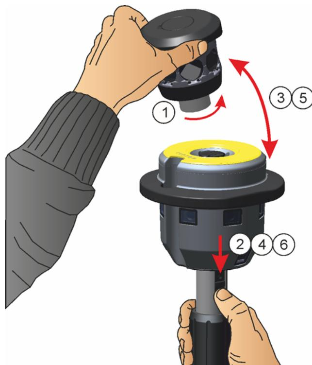
Figure 2.47 Connecting a 360° Prism to the Trimble V10 Imaging Rover
