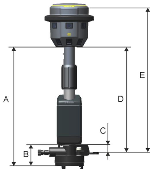
Figure 2.53 Instrument heights on power mount
