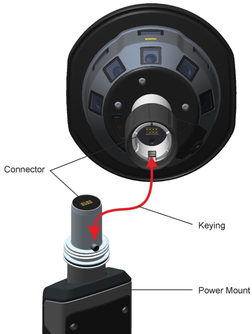
Figure 2.28 Connector and keying on the camera head and power mount
