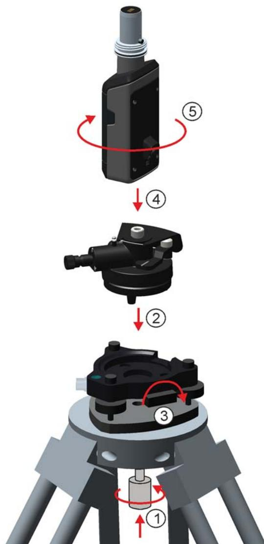
Figure 2.27 High Accuracy Kit assembly
