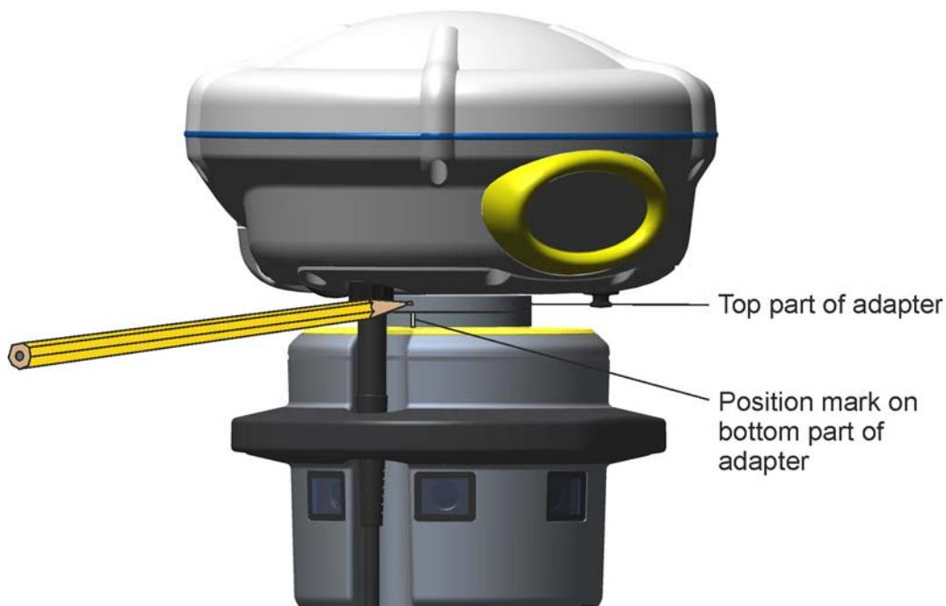
Figure 2.42 Making a reference mark on the top part of the adapter
