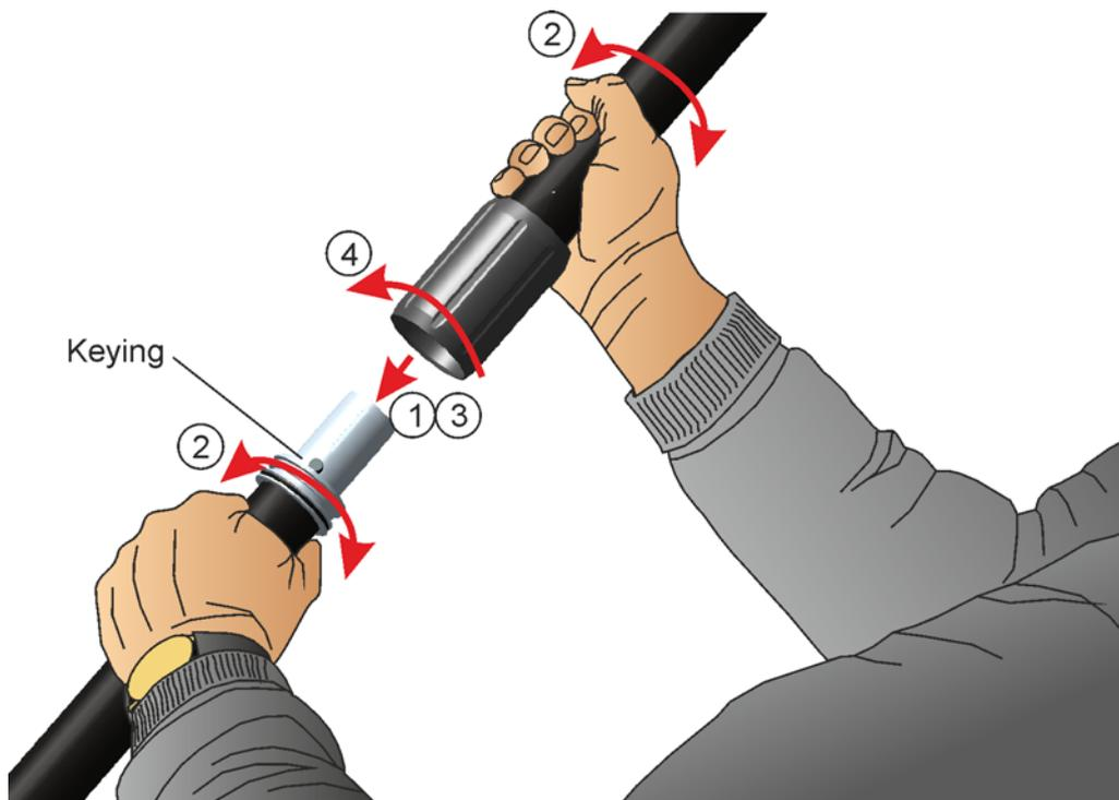
Figure 2.14 Connecting upper and lower Power rod sections
