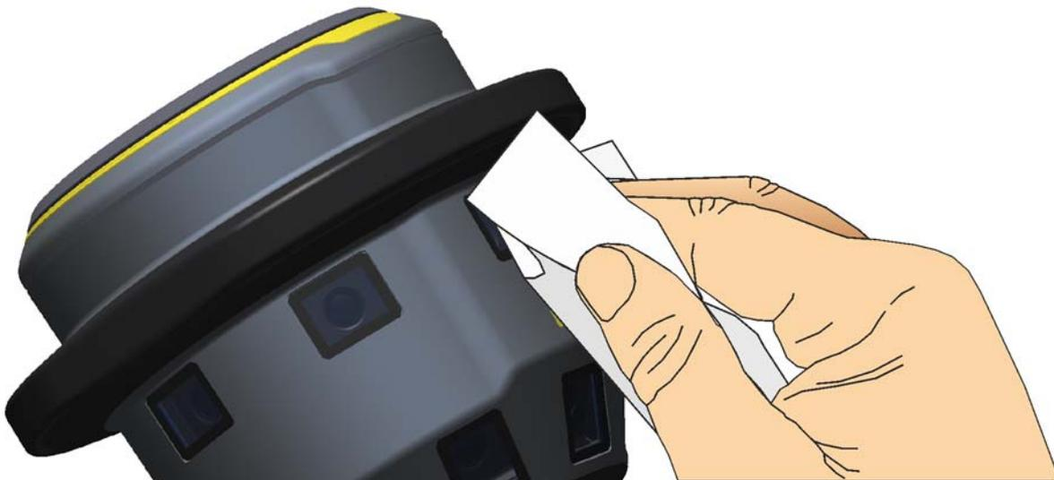
Figure 3.56 Cleaning the instrument windows
